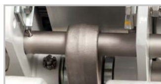
Nickel-plated suspension shaft and suspender
